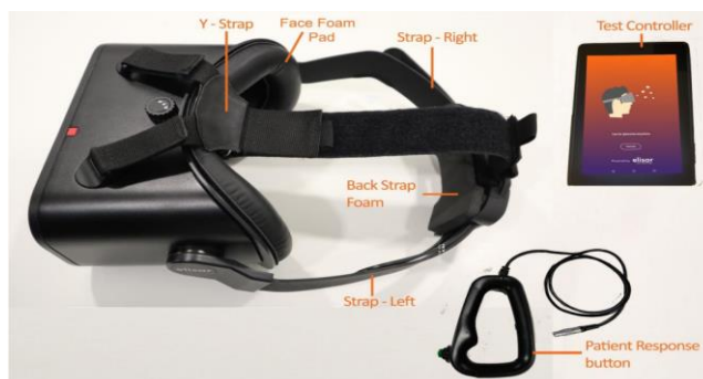
Figure 1: Components of the device, the Elisar Advanced Vision Analyzer . Source: AVA 2022 User Manual.
