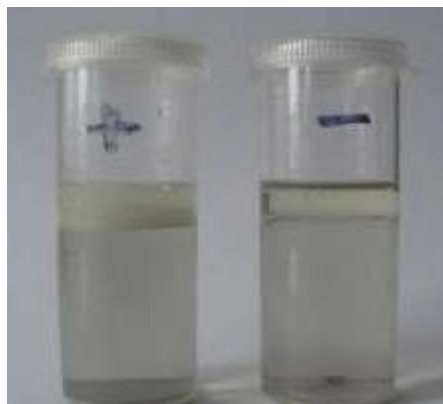
Figure 9. Suspensions formed by intensive mixing of oils with positively charged water do not stratify for hours and, accordingly, retain their milky white or yellowish color (left), unlike suspensions formed by intensive mixing of the same oils with negatively charged water, which stratify within minutes (right); compare with Figure 3.
