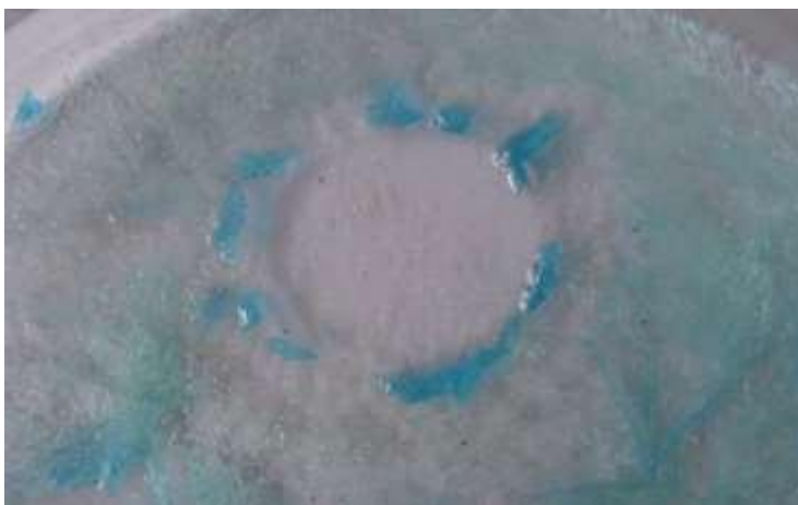
Figure 7: This is how more and less blue crystals are located in the dried solution of copper sulfate, which contained a drop of oil (completely discolored rounded area in the center). A solution of copper sulfate was prepared in uncharged water.
