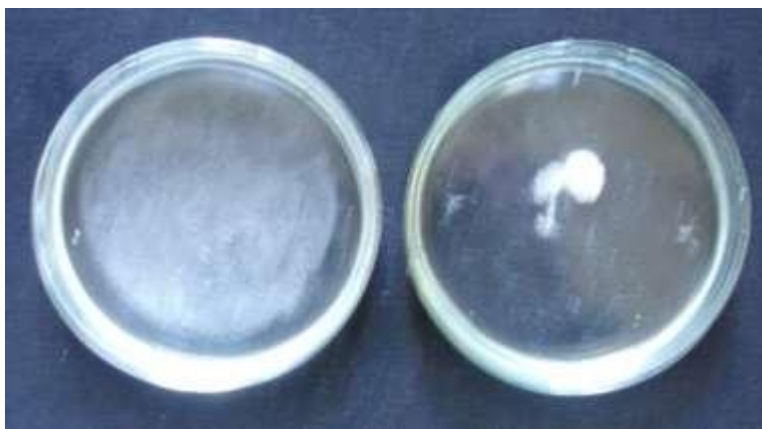
Figure 12. Left: starch powder applied to water with a potential of +250 mV: such water spreads starch powder almost over its entire surface. Right: starch powder applied to water with a potential of -200 mV: starch powder sinks in such water [1, 4].
