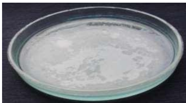
Figure 4. This is a film that has formed from an oil drop on the surface of water with a potential of +500 mV.
