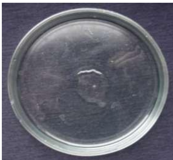
Figure 6. A large oil spot on the surface of water with a potential of -500 mV looks like this; the shape of this spot remains unchanged due to the lack of interaction between the oil and the sufficiently negatively charged water.
