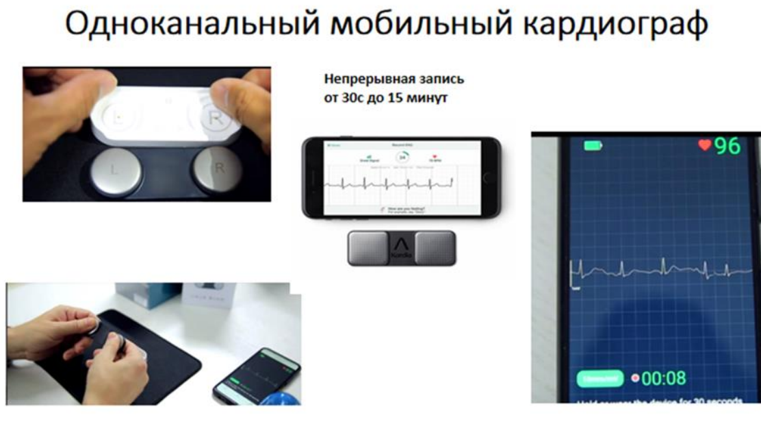
Figure 1: A single-channel mobile cardiograph is used to take an ECG from the fingers, followed by signal transmission via a smartphone to a center for spectral analysis.
